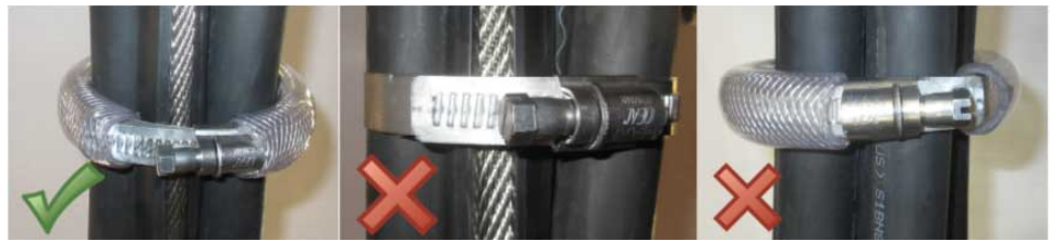
Fig. 18: Installation information for the cable clamps
