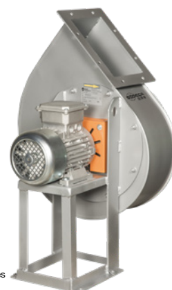
Elastic coupling drive, impeller mounted on the support shaft, mounted on the motor via an elastic coupling. Everything mounted together on a fan pedestal.
