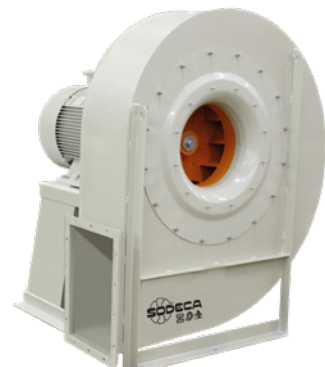
Elastic coupling drive, impeller mounted on the support shaft, mounted on the motor via an elastic coupling. Everything mounted together on a fan pedestal.
