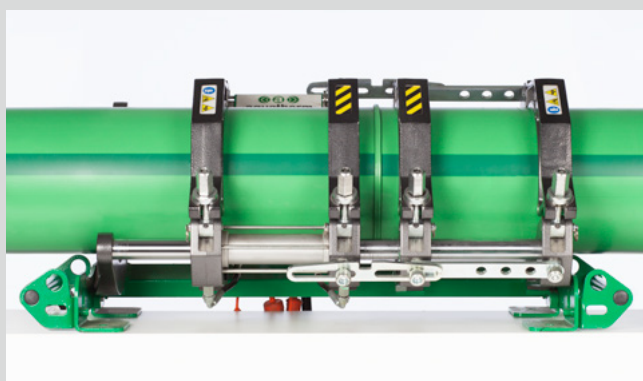
Join the pipes, cool down under pressure
