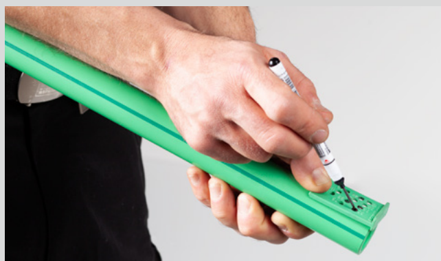
Marking of the welding depth
